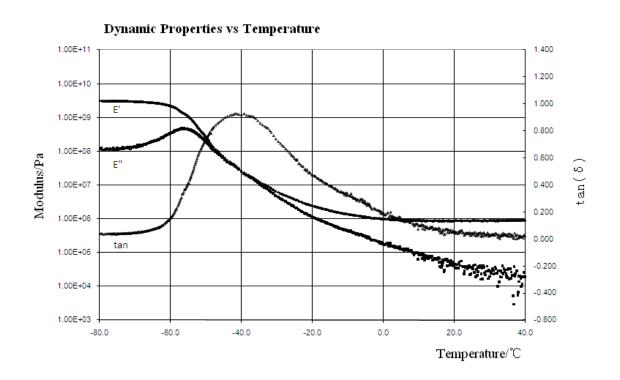
The data contained herein are based on Phichem lab test result and are believed to be reliable. Phichem recommends that the users take test to determine the suitability of a product in particular processing or application/use.
